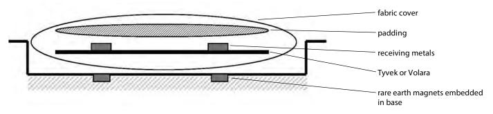
Figure 6. Cross-section of the mitten insert showing the receiving metal and corresponding magnet contact points in the mount base. Illustration: Amanda Harding, © Parks Canada.
