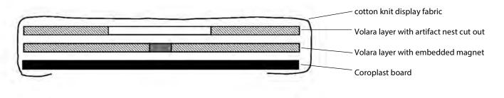
Figure 1. Cross-section of layers making up the mount base. Illustration: Amanda Harding, © Parks Canada.
