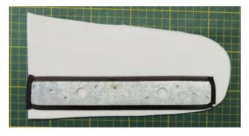
**Figure 5.** Components for mitten insert showing galvanized strap tie, edges covered with black self-adhesive Volara rabbet tape, adhered to Volara. Photo: Amanda Harding, © Parks Canada.
