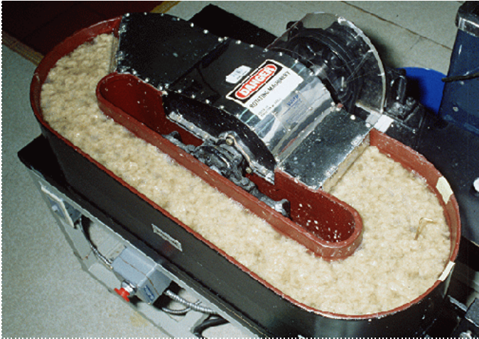
Figure 6. Beating the pulp in the Hollander beater.
