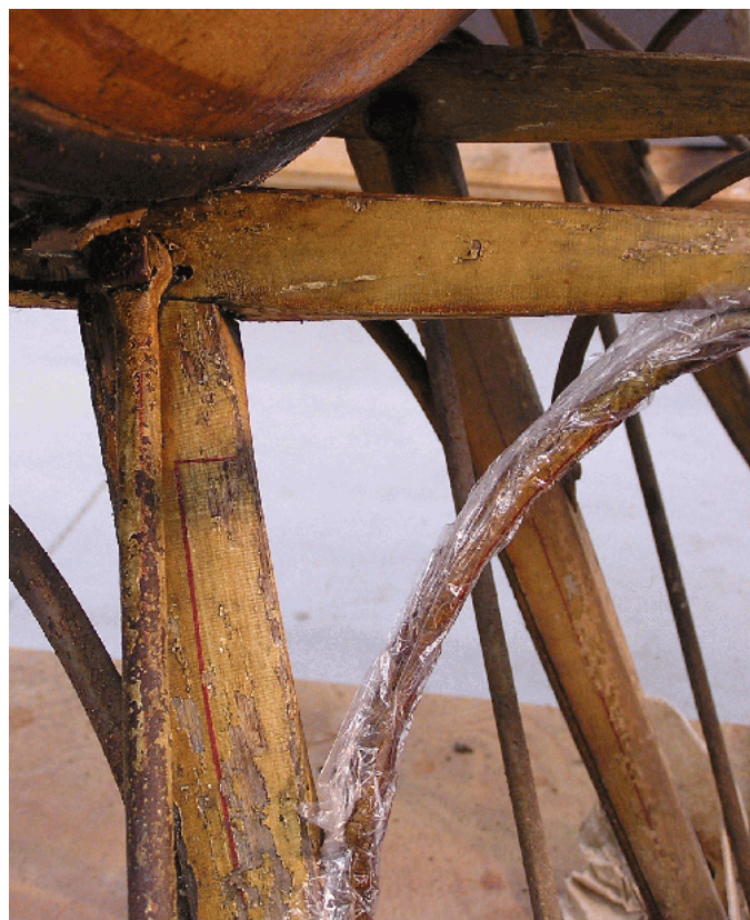
Figure 4. Painted iron component during cleaning with a poultice of 5% citric acid in methyl cellulose. Photograph courtesy of the Canada Science & Technology Museum.
