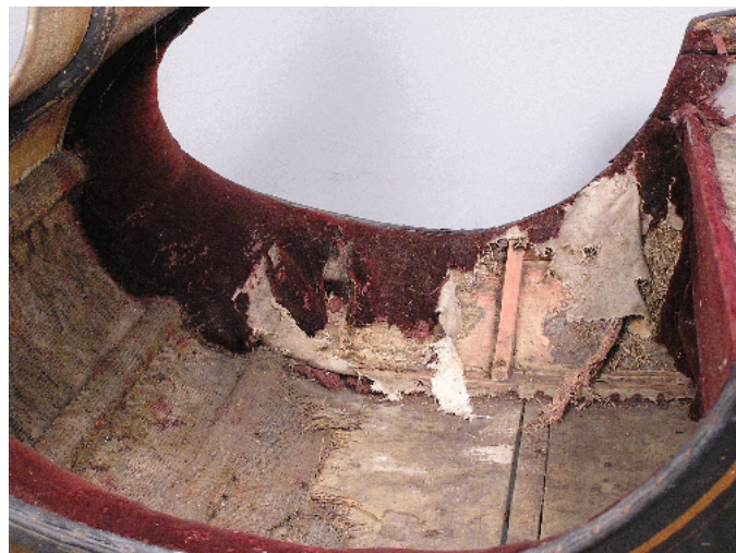
Figure 9. Carpet and plush fabric body-liner before treatment, showing damage from mouse infestation. Photograph courtesy of the Canada Science & Technology Museum.
