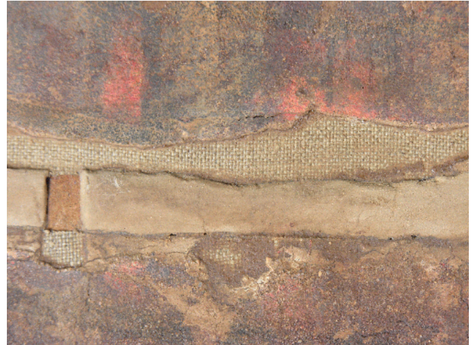
Figure 7. The underlying interleaf linen plus clay-PVA resin filler used by Stout are visible in the joint between two panels. Photo: Courtesy of the Royal Ontario Museum, ©ROM.
