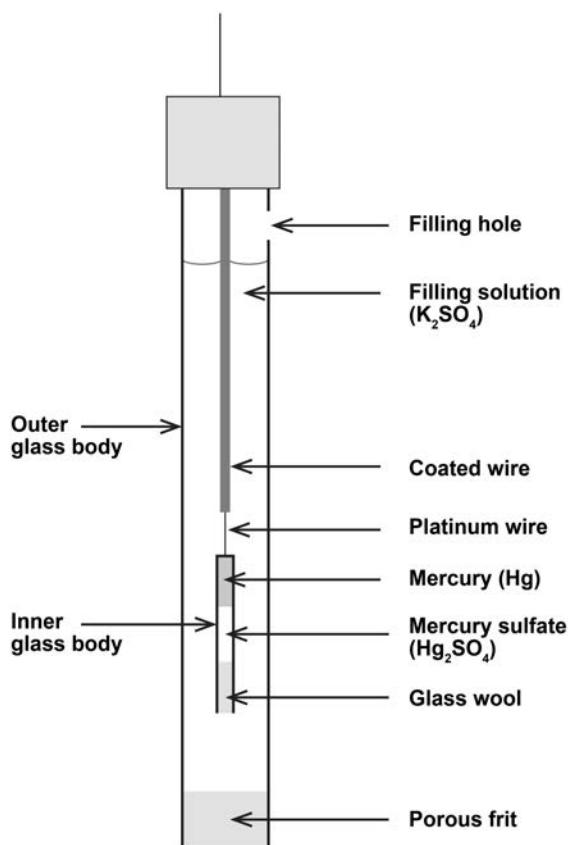
**Figure 2.** Schematic diagram of a saturated mercury-mercury(II) sulfate reference electrode (SSE).
