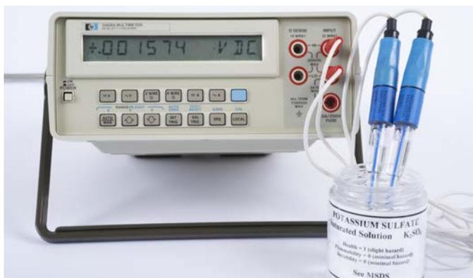
**Figure 4.** Two reference electrodes (one for regular use, one reserved as a control) immersed in an electrolyte (here, saturated potassium sulfate), with the potential measured on a digital voltmeter. The meter reads 0.001574 volts (~1.6 mV).
