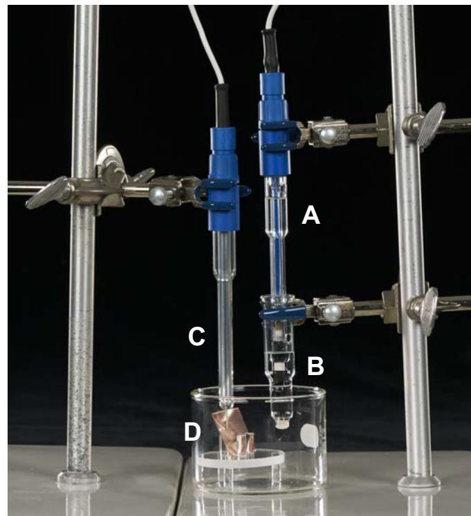
**Figure 6.** Configuration of an electrochemical cell to measure the corrosion potential of copper: (A) reference electrode, (B) salt bridge, (C) platinum electrode and (D) copper sample. For clarity, the electrolyte has not been added to the cell. The container is a 7 cm diameter crystallizing dish.
