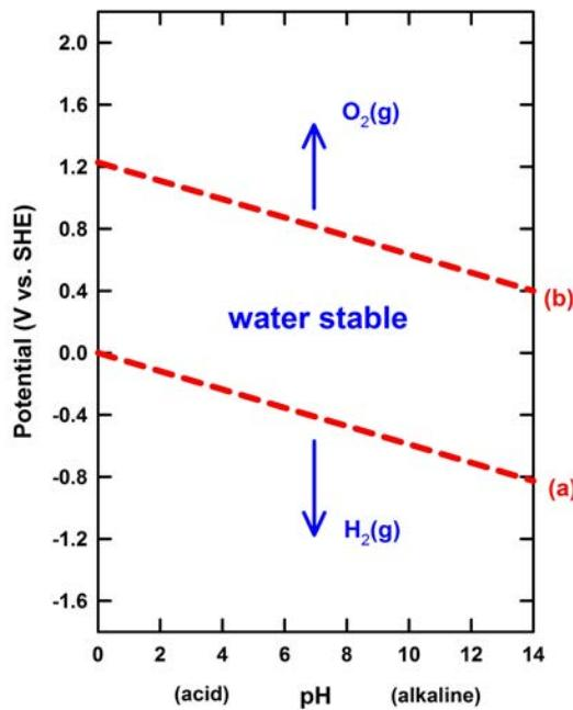
**Figure 11.** Pourbaix diagram showing the stability region of water. For line (a), the potential is given by  $E = 0.000 - 0.059 \text{ pH} - 0.030 \log_{10} p_{\text{H}_2}$ , and for line (b),  $E = 1.228 - 0.059 \text{ pH} + 0.015 \log_{10} p_{\text{O}_2}$ , where the partial pressures  $p_{\text{O}_2}$  and  $p_{\text{H}_2}$  of oxygen and hydrogen are both set equal to 1 atm.
