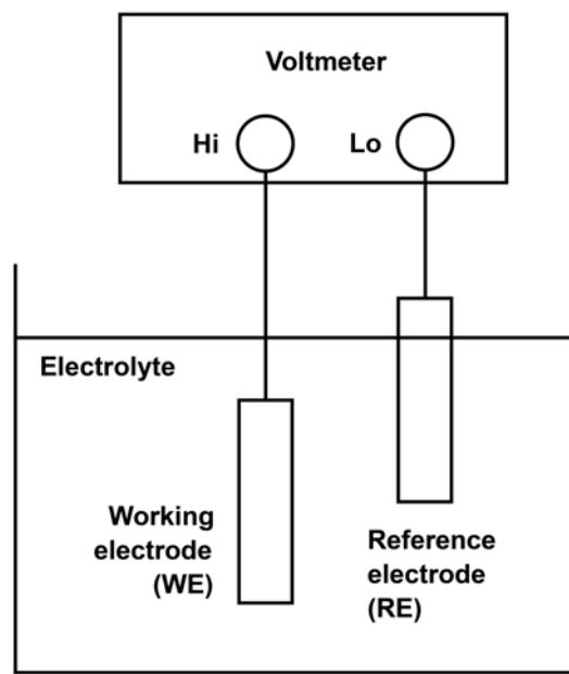
**Figure 1.** Schematic diagram of an electrochemical cell connected to a voltmeter.
