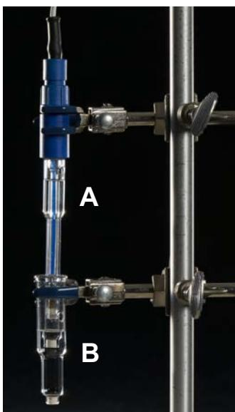
**Figure 3.** Reference electrode (A) and salt bridge (B), held in place with tri-grip clamps attached to the vertical pole of a laboratory stand.
