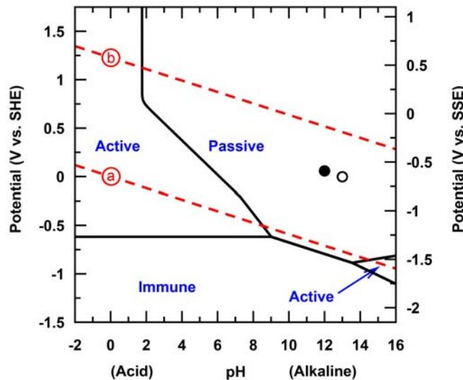
**Figure 10.** Pourbaix diagram for iron, calculated for  $10^{-6} \text{ M}$  concentrations of iron ions. Dashed lines (a) and (b) indicate the stability of water. Solid lines separate Active, Passive and Immune regions. Data points are from corrosion potential measurements made on iron after three hours at pH 12 (solid circle) and pH 13 (open circle) from **Figure 7**.
