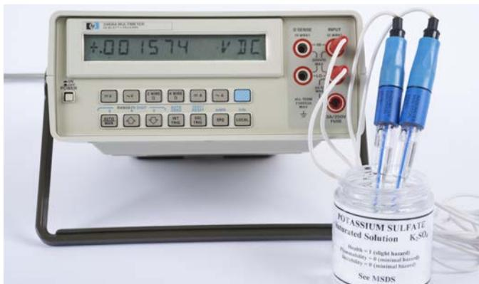
**Figure 4.** Two reference electrodes (one for regular use, one reserved as a control) immersed in an electrolyte (here, saturated potassium sulfate), with the potential measured on a digital voltmeter. The meter reads 0.001574 volts (~1.6 mV).
