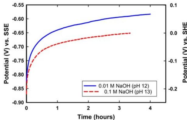
**Figure 7.** Corrosion potential as a function of time for freshly cleaned cold-rolled steel in 0.1 M sodium hydroxide (solid line) or 0.01 M sodium hydroxide (dashed line).
