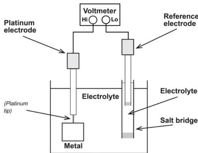
**Figure 5.** Schematic diagram for the measurement of corrosion potential. The platinum tip of the platinum electrode is pushed against the metal to make contact.
