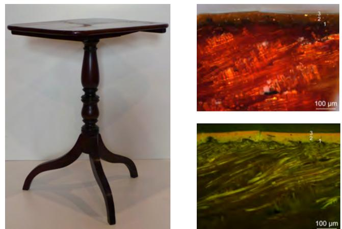
**Figure 14.** (a) Robert Chillas tilt-top table, NBM 2009.38.71. New Brunswick Museum, Saint John, NB. Images of the cross-section: (b) incident light; (c) autofluorescence.
