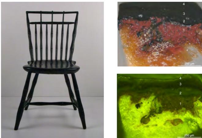
**Figure 11.** (a) Square-back Windsor chair, NBM 2009.25.2. New Brunswick Museum, Saint John, NB. Images of the cross-section: (b) incident light; (c) autofluorescence.
