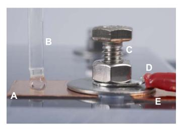
**Figure 8.** Measuring the corrosion potential of a copper sample (A) using a local measurement. Components include: (B) salt bridge, (C) nut and bolt, (D) ring terminal and (E) copper spacer.
