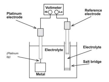
**Figure 5.** Schematic diagram for the measurement of corrosion potential. The platinum tip of the platinum electrode is pushed against the metal to make contact.
