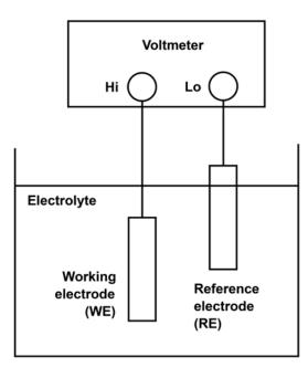
**Figure 1.** Schematic diagram of an electrochemical cell connected to a voltmeter.
