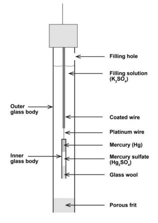
**Figure 2.** Schematic diagram of a saturated mercury-mercury(I) sulfate reference electrode (SSE).
