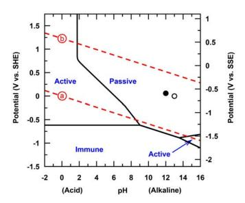
**Figure 10.** Pourbaix diagram for iron, calculated for 10<sup>-6</sup> M concentrations of iron ions. Dashed lines (a) and (b) indicate the stability of water. Solid lines separate Active, Passive and Immune regions. Data points are from corrosion potential measurements made on iron after three hours at pH 12 (solid circle) and pH 13 (open circle) from **Figure 7**.
