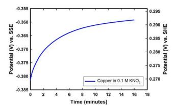
**Figure 9.** Corrosion potential as a function of time for freshly cleaned copper using a local measurement. The electrolyte was 0.1 M potassium nitrate.
