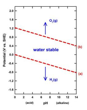
**Figure 11.** Pourbaix diagram showing the stability region of water. For line (a), the potential is given by  $E = 0.000 - 0.059 \text{ pH} - 0.030 \log_{10} p_{H2}$ , and for line (b),  $E = 1.228 - 0.059 \text{ pH} + 0.015 \log_{10} p_{O2}$ , where the partial pressures  $p_{O2}$  and  $p_{H2}$  of oxygen and hydrogen are both set equal to 1 atm.
