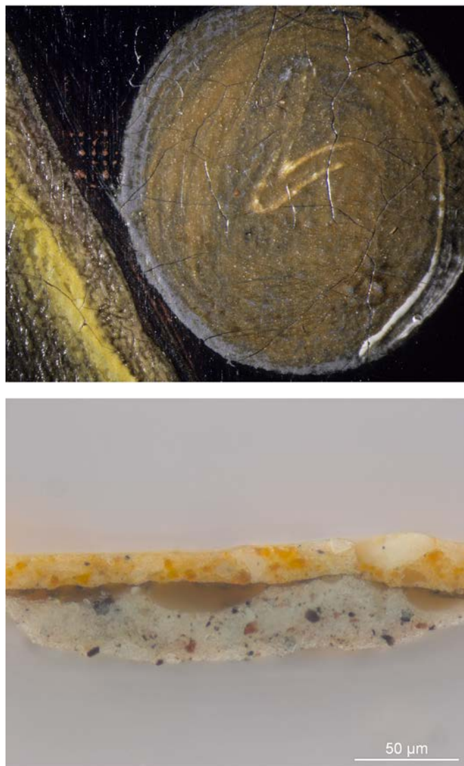
Figure 12. Top button on jacket, portrait of James McGill. Top: photographic detail of button showing grey paint with overlying yellow paint. Bottom: cross-section showing varnish between grey and yellow layer. Photos: © Government of Canada, Canadian Conservation Institute.
