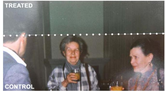
**Figure 6.** An example of colour difference between the treated and control samples (separated by a dotted line) that was visible to the eye (Print #13). The treated sample showed a greener hue ( $-\Delta a^*$ ).
