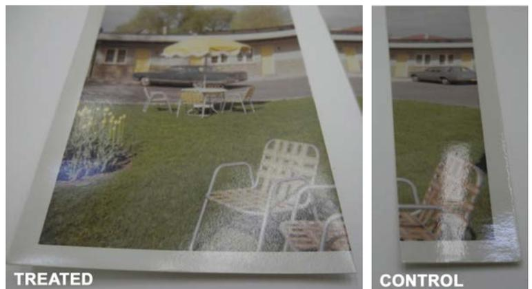
**Figure 7.** Surface sheen difference between treated and control samples (Print #38).
