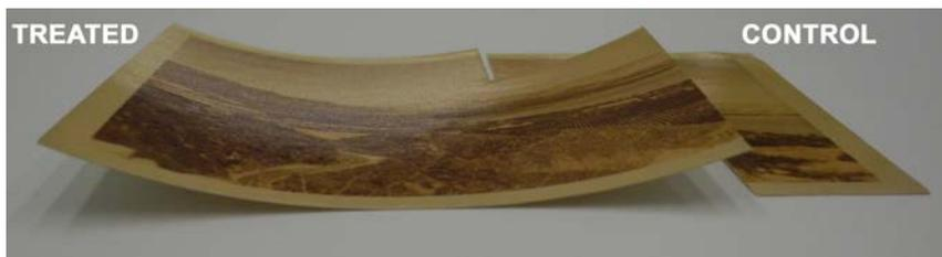
**Figure 8.** Difference in planarity (strong curling) between treated and control samples (Print #55).
