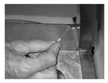
**Figure 1.** Sampling the underside of the rear seat rail of a chair, an example of a location on a piece of furniture where original finish may remain.
