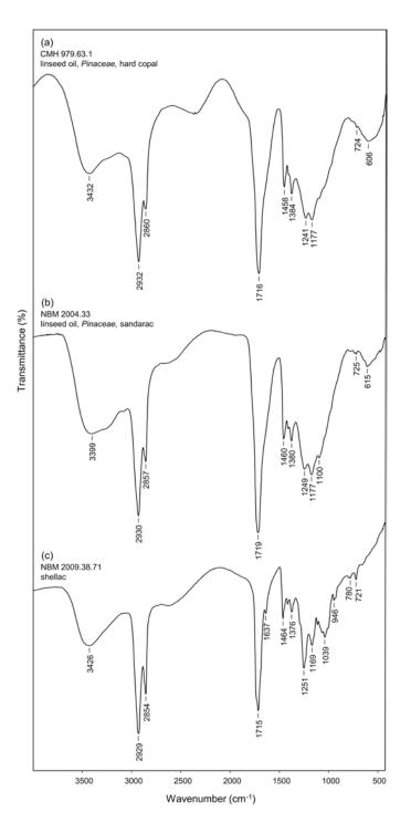
**Figure 7.** Infrared spectra of furniture finish samples: (a) slant top desk (CMH 979.63.1); (b) chair (NBM 2004.33); (c) tilt-top table (NBM 2009.38.71).
