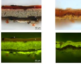
Figure 12. Incident light and autofluorescence images of the crosssections prepared from left: the finish on the side chair (NB 984.4.2.b); and right: the finish on the secretary (NB 983.11).
