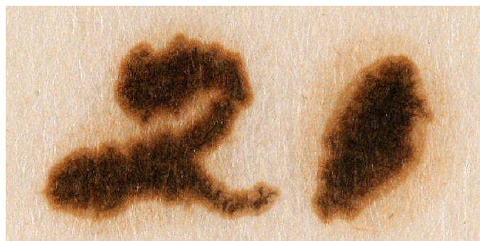
Figure 6c. An example of the ‘haloing’ effect of the sulphuric acid as it migrates into the paper appearing as a discoloration around the ink line.
