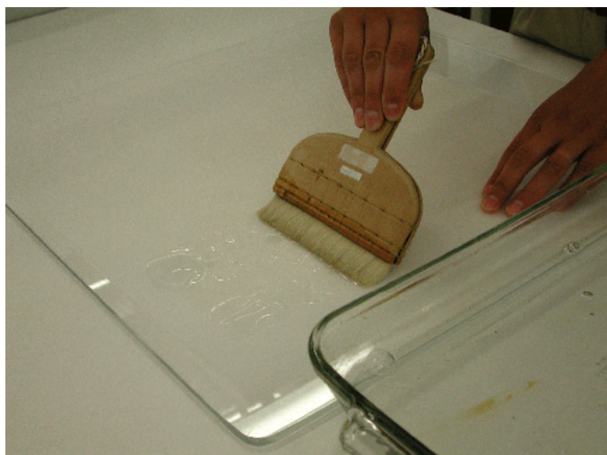
Figure 7. Creating the Klucel G coated RK-0 tissue by brushing prepared Klucel G over RK-0 tissue covered with a fibreglass screen.
