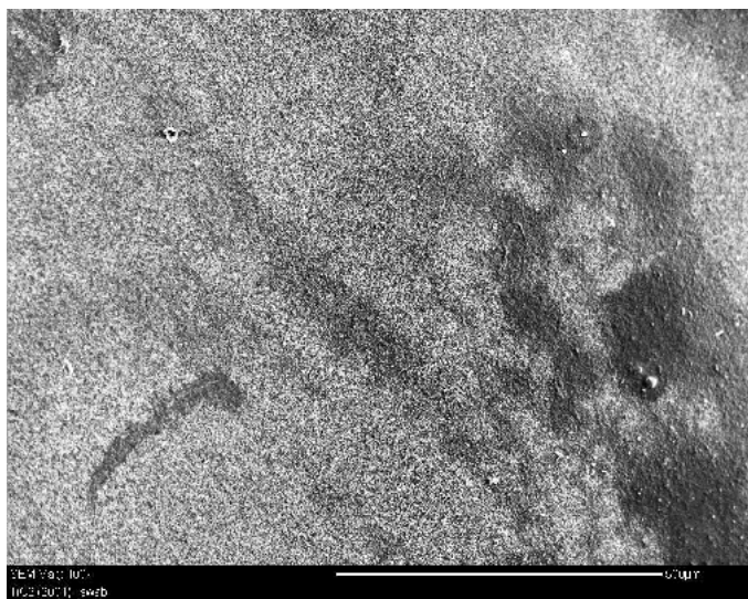
Figure 7. Scanning electron micrograph of swabbed titanium white sample with areas of displaced additives (cast in 2001), at 100x magnification. Scale: 1 cm = 125 μ.
