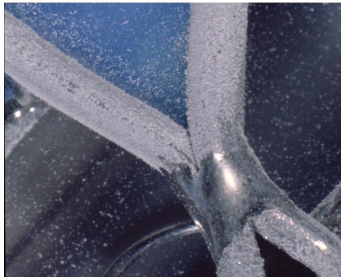
Figure 2. A close-up of a soft solder join in the stained glass angel pictured in Figure 1, which shows that the solder is not corroding. It is probably a lead-tin alloy with sufficient tin to make it more resistant to active corrosion than the adjacent lead came. Photograph courtesy of the Canadian Conservation Institute.
