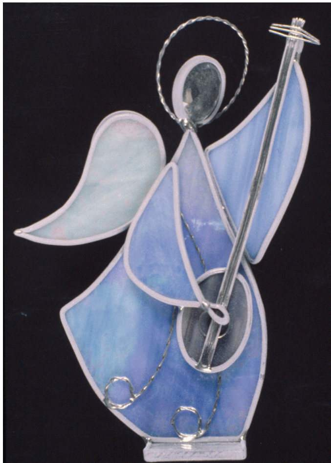
Figure 1. This stained glass angel was stored in a closed wooden cabinet; the lead came surrounding the glass is suffering from active corrosion, and has turned white. Photograph courtesy of the Canadian Conservation Institute.
