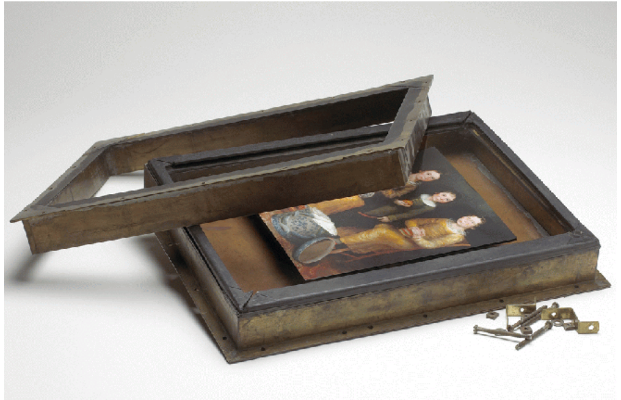
Figure 5. An example of the sealed micro-climate metal boxes introduced to protect wood-panel paintings by George Harbour and H. E. Thompson, early 1928. The box contains a reduced copy of the painting The Perras Children 1823, by an unknown American artist, in the collection of the National Gallery of Canada, ID # 9057. The front glass is not shown, nor is the Beaverboard as humidity buffer. Photograph © and courtesy of the National Gallery of Canada Library and Archives, Ottawa.
