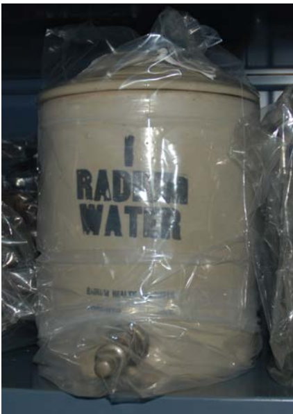
Figure 1b. Radium water jar; Cat. # 2002.0538; Radiation level at 25 cm: 60 \mu\text{Sv/hr} ; Annual limit: 16.67 hr/yr.
