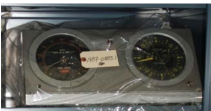
Figure 1c. Wind speed & direction indicator; Cat. # 1987.0783; Radiation level at 25 cm: 120 \mu\text{Sv/hr} ; Annual limit: 8.3 hr/yr.
