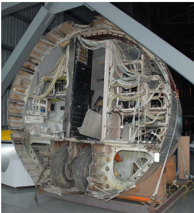
Figure 2. Luminous placards in nose section of Comet Aircraft which give readings over 400 \mu\text{Sv/hr} at 15 cm from the surface. Moving to 30 cm reduces the readings to 100 \mu\text{Sv/hr} . Photograph © and courtesy of the Canada Science & Technology Museum Corporation.
