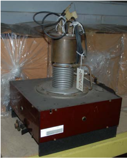
Figure 1a. Spectrophotofluorimeter; Cat. # 1988.0672; Radiation level at 25 cm: 80 \mu\text{Sv/hr} ; Annual limit: 12.5 hr/yr.
