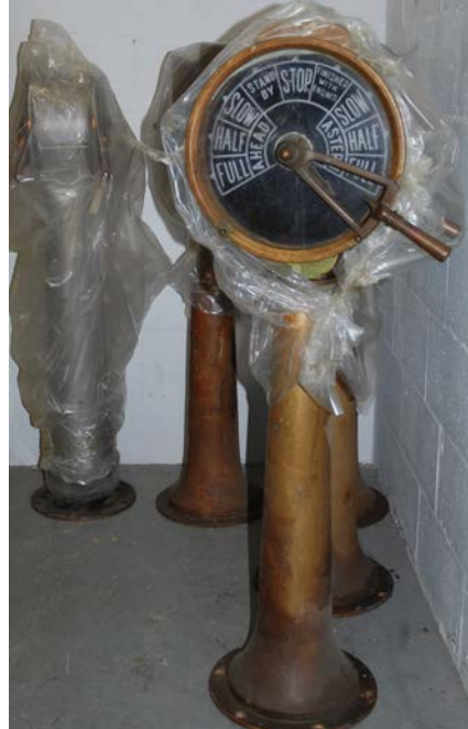
Figure 1d. Ship's telegraph; Cat. # 1971.0688; Radiation level at 25 cm: 75 \mu\text{Sv/hr} ; Annual limit: 13.3 hr/yr.
