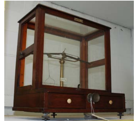
Figure 1g. Analytical balance; Cat. # 1969.1002; Radiation level at 25 cm: 120 \mu\text{Sv/hr} ; Annual limit: 8.3 hr/yr.
