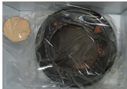
Figure 1f. Aviation magnetic compass; Cat. # 1970.0662; Radiation level at 25 cm: 300 \mu\text{Sv/hr} ; Annual limit: 3.3 hr/yr.
