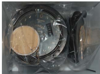
Figure 1e. Altimeter; Cat. # 1970.0809; Radiation level at 25 cm: 90 \mu\text{Sv/hr} ; Annual limit: 11.1 hr/yr.
