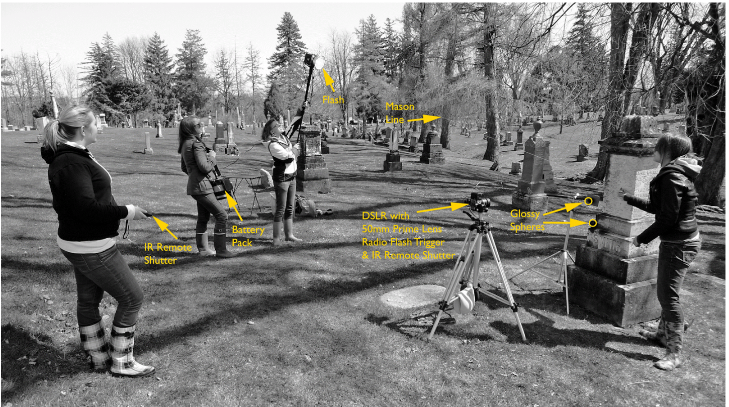
Figure 6a. RTI field set-up in action in the Cataraqi Cemetery, Kingston, Ontario with a group of students learning the technique. The RTI equipment is labelled.
