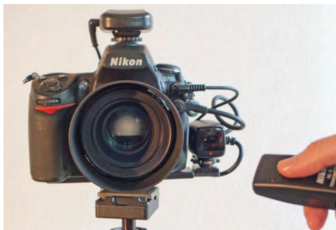
Figure 4. Complete Nikon D700 camera with a 50mm lens and flash and shutter remotes mounted on a ball-head.
