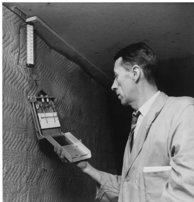
Figure 4. Mervyn Ruggles monitoring the temperature and relative humidity inside the truck used by W. Sparks & Son Ltd. to move the collections, in November 1959. Credit: Rosemary Gilliat Eaton/National Gallery of Canada Library and Archives/ Record Number: 090253. Photograph courtesy of the National Gallery of Canada Library and Archives, Ottawa.
