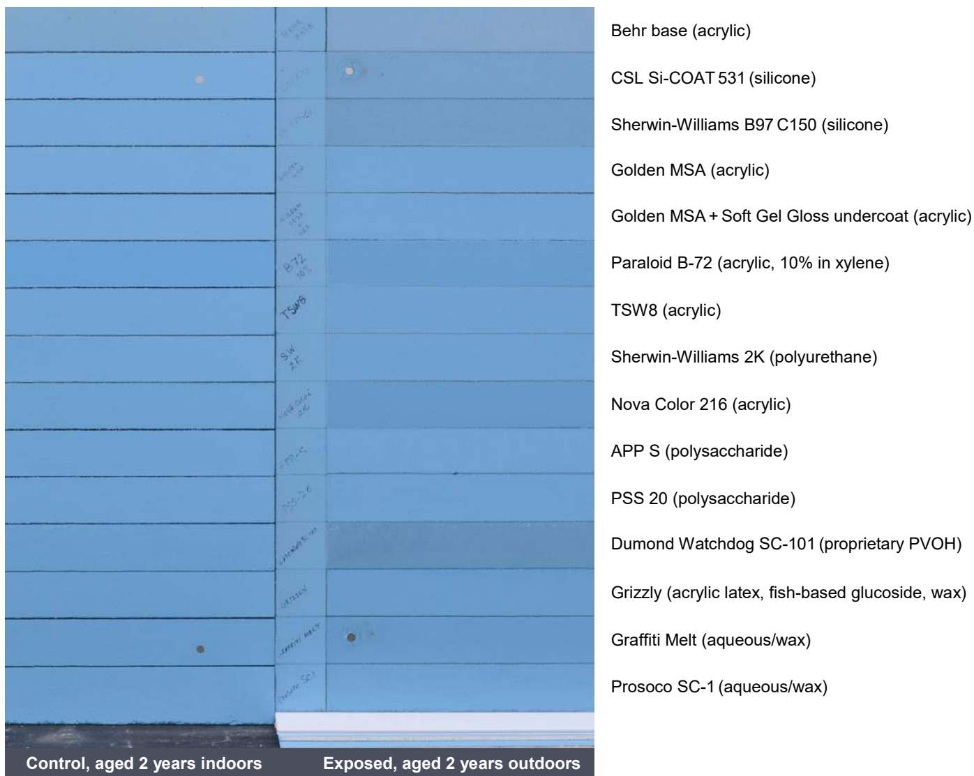
Figure 3. Comparison of the indoor control (left) and the exposed (right) sample panels viewed side by side in 2015 after two years of ageing.
