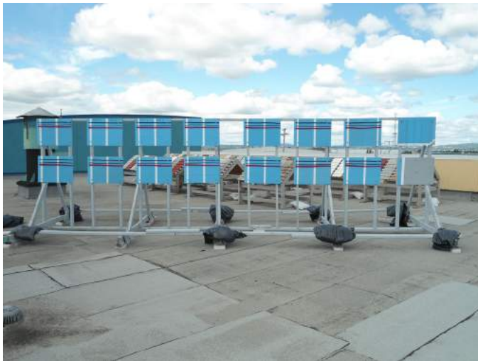
Figure 1. Outdoor exposure rack in 2015, before graffiti removal. Blue and white painted panels (vertical bands) have been marked with black, silver and red graffiti (horizontal markings). The unmarked, upper right sample strip panel comprises all the coatings and was used for gloss and colour measurements. The lower right Magnesiacore panel consists of two thin vertical bands of uncoated blue and white paint on a grey background.
