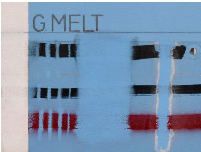
Graffiti Melt temporary anti-graffiti coating (6 layers)
