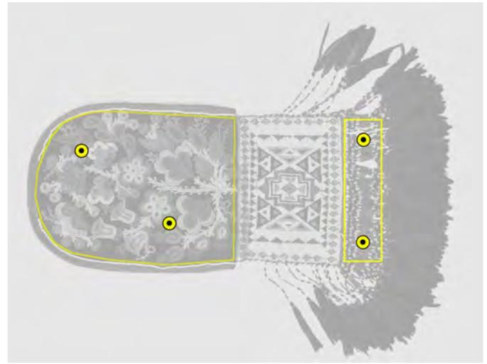
**Figure 4.** Fire bag, verso. The yellow rings with black centres indicate the location of the washers that correspond with the magnets in the base. The yellow outlines indicate the location of the receiving metal layers: layer inserted in pouch on left and twill tape sewn on the back on the right. The verso of the bag is placed face down in the mount. Photo: Amanda Harding, © Parks Canada.
