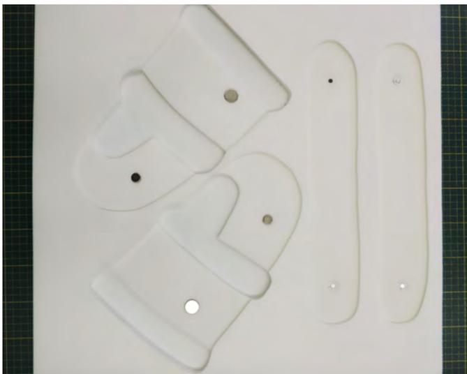
**Figure 2.** Mount base showing rare earth magnets embedded in Volara layer and nested layers of Volara to accommodate the thickness of the objects. Photo: Amanda Harding, © Parks Canada.
