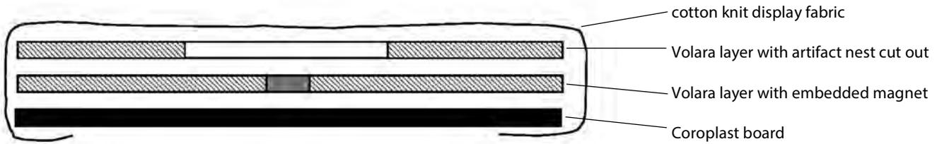
**Figure 1.** Cross-section of layers making up the mount base. Illustration: Amanda Harding, © Parks Canada.
