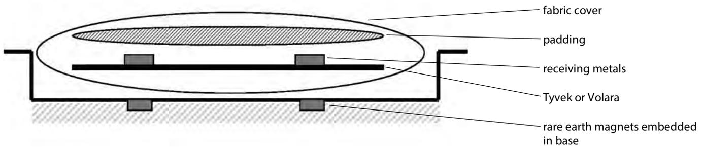
**Figure 6.** Cross-section of the mitten insert showing the receiving metal and corresponding magnet contact points in the mount base. Illustration: Amanda Harding, © Parks Canada.
