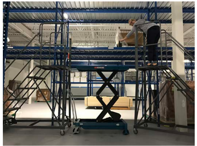
Figure 2. KLETON scissor lift being used in conjunction with ladders on either side.
