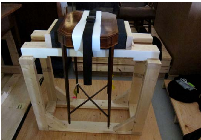
Figure 19. An example of a custom table mount screwed directly onto a pallet.
