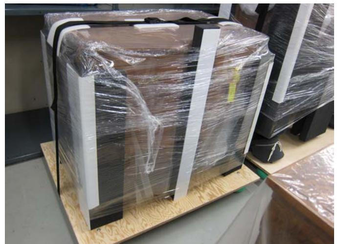
Figure 18. An example of a fully wrapped and palletized chest of drawers with reinforced corners ready for shipment.
